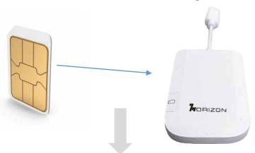
Plug in Dongle, and Wait 40 sec to boot, Check Ethernet network is active
